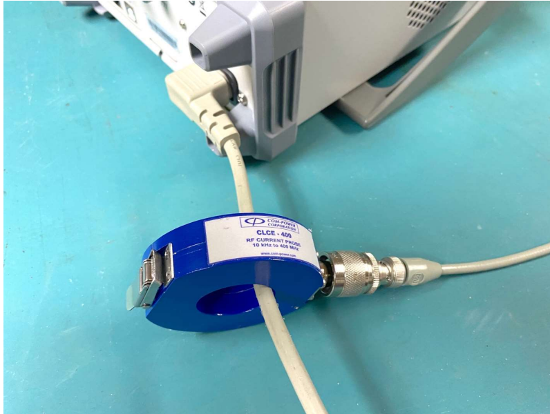
Figure 8: Com-Power CLCE-400 RF current probe measuring line cord common-mode harmonic emissions on a product under test.
